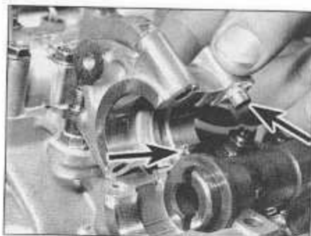
11.34b ... then refit to cylinder head, ensuring locating dowels are in position (arrowed)
