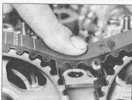
9.11 On DOHC engines, push on upper run of timing belt midway between camshaft pulleys to relieve timing belt tension
