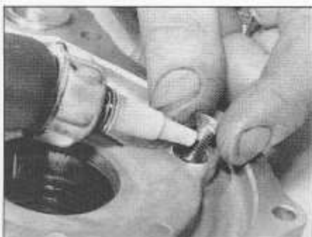
16.12 Apply thread-locking compound to pump cover screws and tighten to specified torque
