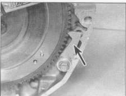
19.2 Use fabricated tool (arrowed) to lock flywheel/driveplate
