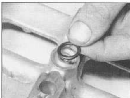
18.16a Fit a new O-ring to the recess in the main bearing cap bridge ...
