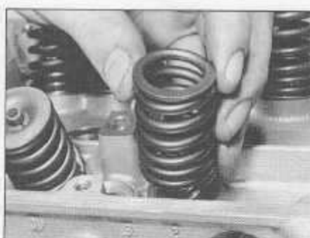
8.3a Fit the valve spring, ensuring its closest-wound coils are at the bottom ...
