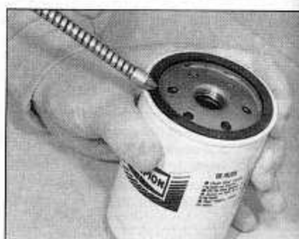
9.9 Apply a light coating of clean oil to the oil filter sealing ring before fitting
