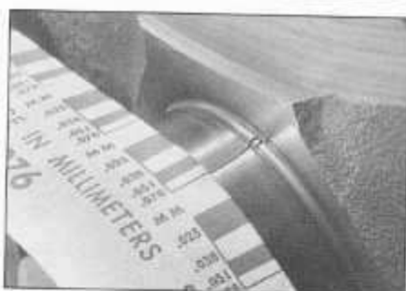
17.12 Use the scale provided to check the width of the crushed Plastigauge (at its widest point), giving bearing running clearance
