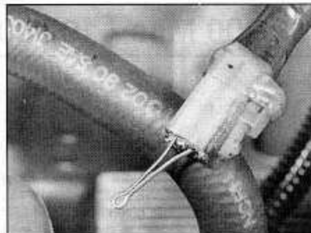
37.6 Using a split pin to connect the ignition timing adjuster terminals together
