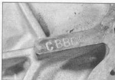
18.3 Cylinder block main bearing journal identification letters. Left-hand letter is for No 1 bearing, right-hand letter for No 5 bearing
