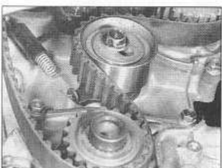
8.9 Timing belt lower run (viewed from underneath)
