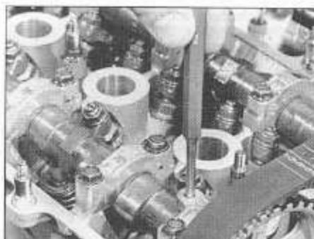
8.2c On DOHC engine, peg camshafts in position to prevent movement under valve spring pressure when timing belt is removed
