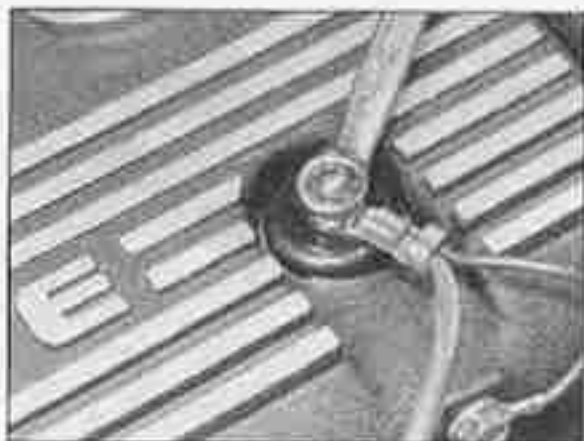
5.11a On SOHC engine, do not forget to fit earth lead beneath left-hand front cover retaining nut
