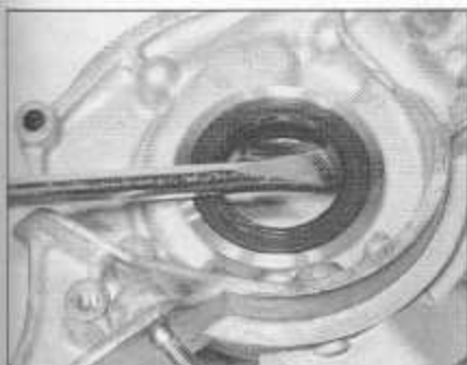
16.10a Removing oil pump seal with a flat-bladed screwdriver ...
