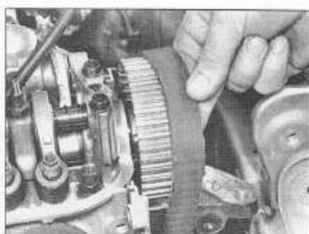
8.6b ... to allow timing belt to be fully removed from engine
