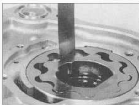
16.6b Measuring oil pump rotor tip clearance
