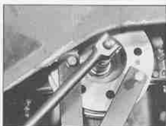
6.5 Using fabricated tool to retain crankshaft pulley while retaining bolt is slackened
