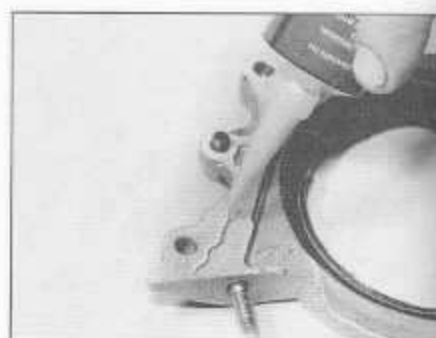
18.13 Apply sealant to oil seal housing mating surface ...
