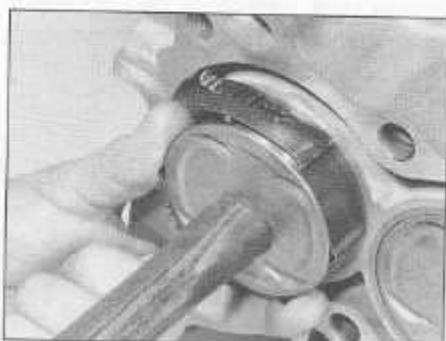
17.19c Use a piston ring compressor to clamp rings in position, then gently tap pistons into cylinder bores
