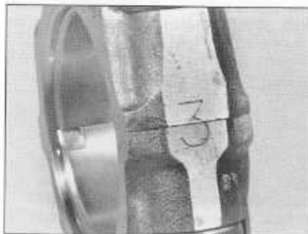
17.2 Connecting rod big-end journal identification number
