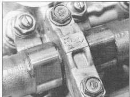
11.33 Use identification marks to ensure all camshaft bearing caps are correctly positioned on refitting
