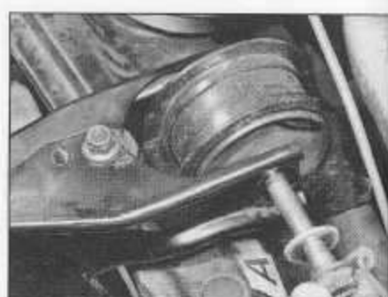
20.22b . . . then undo mounting through-bolt and withdraw mounting bracket - manual gearbox shown
