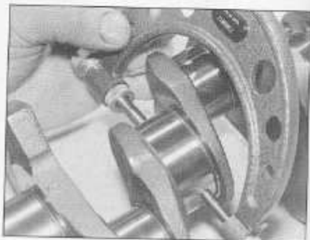
13.8b Measuring the diameter of a crankshaft journal
