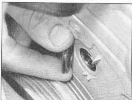
8.15a Remove rubber grommet from timing belt lower cover to gain access to tensioner pulley bolt
