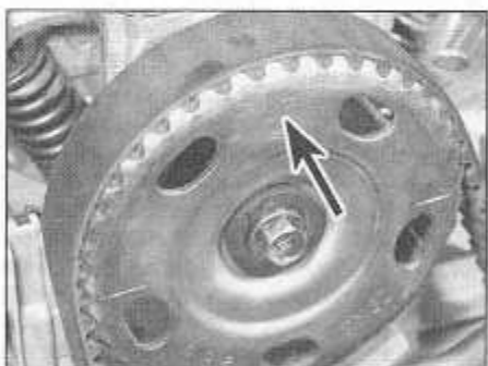
8.8a On SOHC engine, ensure UP mark on camshaft sprocket (arrowed) is at top ...
