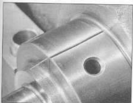
17.11 Lay length of Plastigauge on journal to be measured, parallel to crankshaft centre-line
