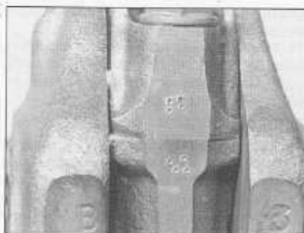
10.9 Always mark big-end caps and connecting rods prior to removal
