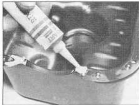
14.10 Apply sealant to sump and gasket upper surface on either side of crankshaft cut-outs
