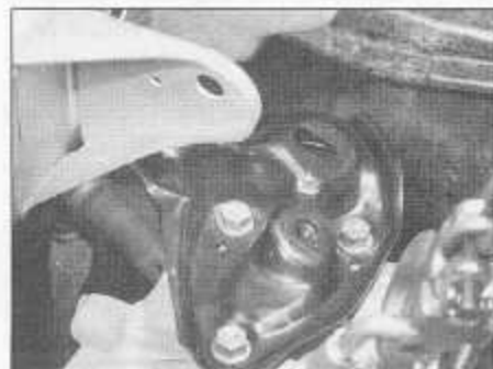
20.7c Right-hand mounting plate is retained by three bolts
