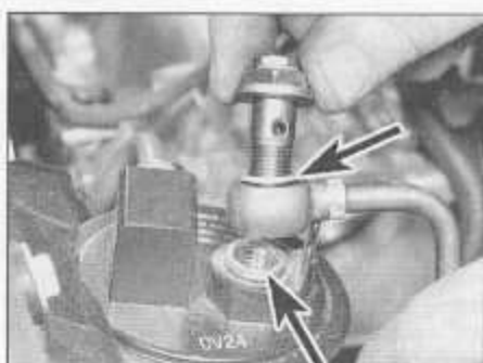
4.14a Disconnect the outlet hose from the fuel filter. Note sealing washers (arrowed)
