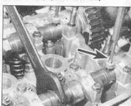
9.12 Using an open-ended spanner, return camshafts to original positions and peg them in place with a suitable tool (arrows)
