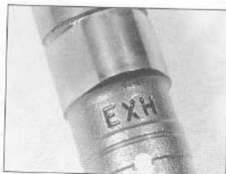
11.15 On DOHC engines, camshafts are marked to avoid confusion - exhaust camshaft shown
