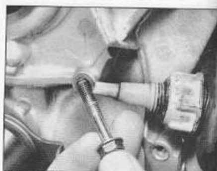
15.8 Apply thread-locking compound to oil pump bolts and tighten to specified torque
