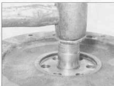
19.5 Tap flywheel centre bearing into position using a hammer and suitable tubular drift
