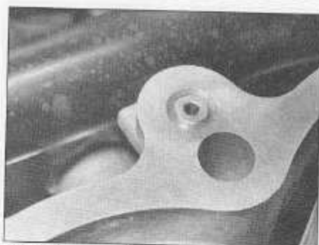
13.12 Remove oil control jet from cylinder block, noting which way around it is fitted
