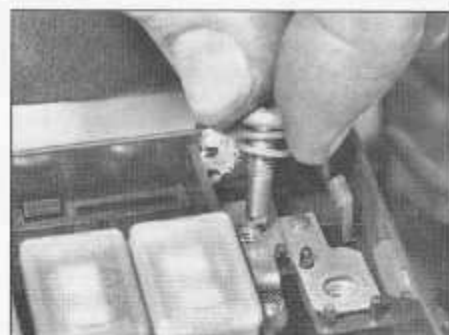
4.12 Undo the retaining screw and disconnect the battery lead to the fusebox terminal
