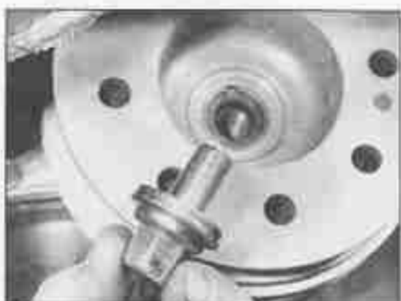
6.7b Refitting crankshaft pulley retaining bolt and special washer
