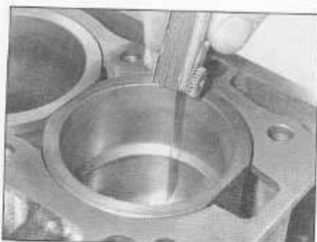
12.5b Measuring piston ring end gap
