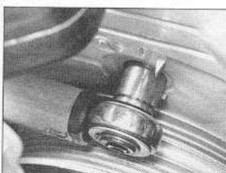
8.15b Tension timing belt then tighten tensioner pulley bolt to specified torque
