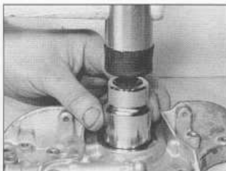
16.10b ... and tapping new seal into position using a suitable tubular drift
