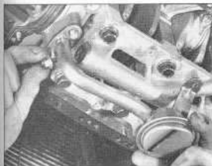
14.8 Unbolt oil pump pick-up pipe/strainer and remove from engine
