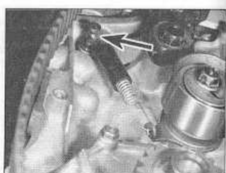
9.34b ... and spring is correctly located on pillar bolt (arrowed)
