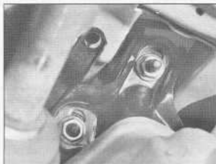
20.7b ... and two mounting plate retaining nuts (viewed from underneath)
