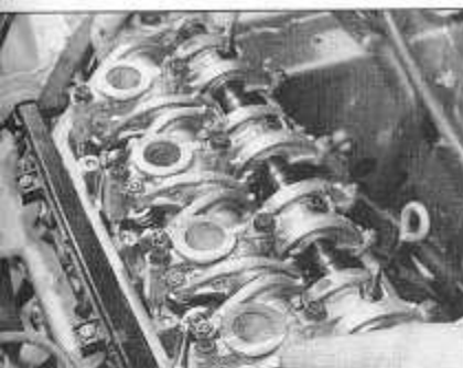
11.6 On SOHC engines, remove camshaft bearing cap/rocker arm assembly ...
