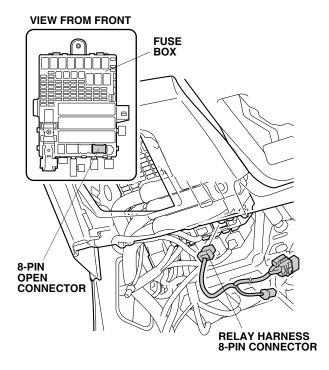
NOTE: If the 8-pin connector is already used by another accessory, locate the 8-pin connector taped to that other accessory harness. Remove the tape and dummy connector from that other accessory harness. Plug the fog light harness 8-pin connector into that other accessory harness.
