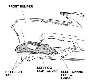
12. Install the left fog light to the front bumper with two 5 x 14 mm self-tapping screws and one self-tapping screw removed in step 10.
