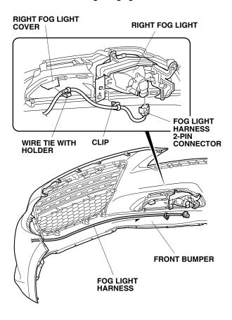
18. Attach the clip to the right fog light. Install a wire tie with holder to the fog light harness, and attach it to the right fog light cover.
