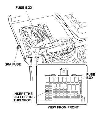
37. If an option fuse 20A label is already attached to the fuse box cover, go to step 38. If not, use isopropyl alcohol on a shop towel to thoroughly clean the fuse box cover where the fuse label will attach. Attach the 20A fuse label to the fuse box cover at the location shown.
