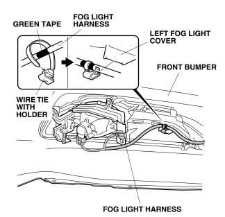
17. Route the other fog light harness 2-pin connector to the right side of the front bumper, and plug the 2-pin connector into the right fog light.
