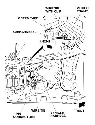
23. Secure the 1-pin connectors to the vehicle harness with one wire tie.
