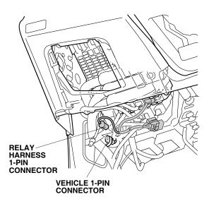
Remove the lower hood opener bolt. Secure the relay bracket to the vehicle panel with the hood opener bolt.
