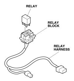
26. Plug the relay harness 8-pin connector into the open 8-pin connector in the fuse box.
