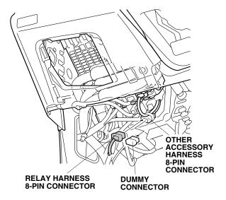
27. Plug the relay harness 1-pin connector into the vehicle 1-pin connector.
