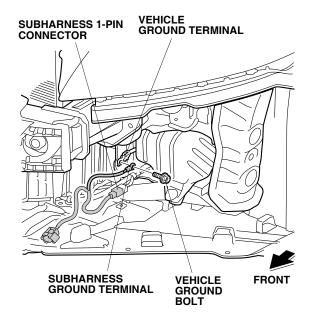
22. Install a wire tie with clip to the subharness at the green tape. Insert the wire tie with clip into the hole in the vehicle frame.
