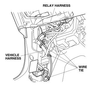
32. Turn the steering wheel counterclockwise. Unplug the vehicle harness connector from the light switch.
