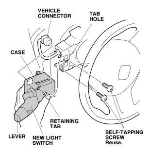
35. Plug the vehicle connector into the new light switch.
