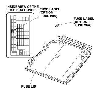
38. Using isopropyl alcohol on a shop towel, thoroughly clean the fuse box cover where the blank fuse label will attach. Attach the fuse label to the fuse box cover at the location shown.
