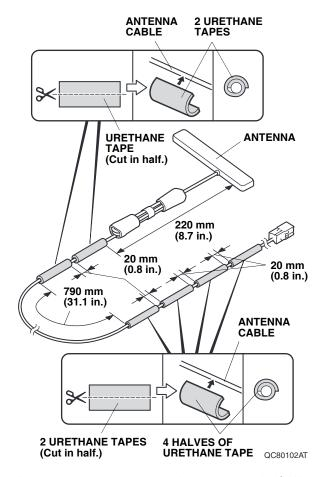
29. Using scissors, cut two urethane tapes in half. Wrap four halves of urethane tape around the antenna cable at the measurements shown.
