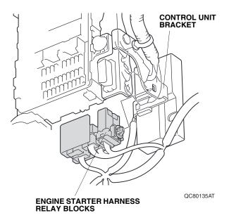
49. Align the white tape on the engine starter harness with the clip on the vehicle harness, and secure the engine starter harness to the vehicle harness using one wire tie.
