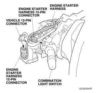
77. Align the white tape on the engine starter harness with the clip on the vehicle harness, and secure the engine starter harness to the vehicle harness with one wire tie. Secure the engine starter harness 12-pin connector to the vehicle frame with one wire tie. Do not secure it to the SRS harness.
