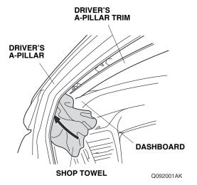
13. Remove the driver's A-pillar trim from the upper clip (unplug the vehicle connector, if equipped). Carefully remove the shop towel and any clips that fell from the driver's A-pillar trim.
