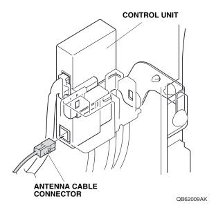
56. Using one wire tie, secure the antenna cable and engine starter harness to the vehicle harness.
