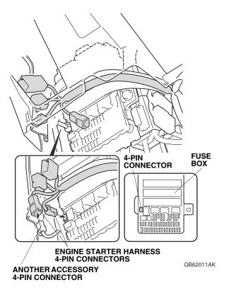
62. Using one wire tie, secure the engine starter harness 4-pin connector to the vehicle harness.
