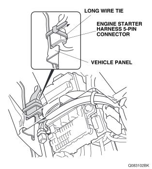
67. Route the engine starter harness as shown. Using one wire tie, secure the engine starter harness at the white tape to the hole in the dashboard panel.
