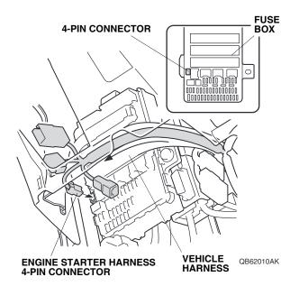
61. Plug the engine starter harness 4-pin connector into the fuse box.
