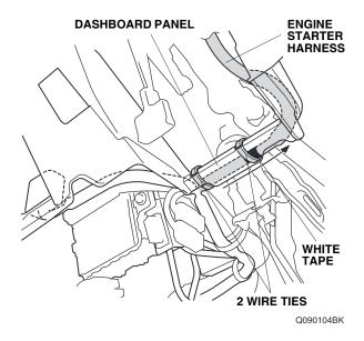
68. Using one wire tie, secure the engine starter harness to the hole in the dashboard panel.
