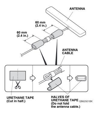
28. Using scissors, cut one urethane tape in half.
