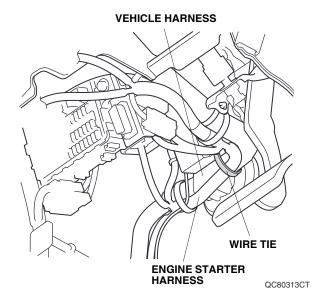
60. Route the engine starter harness along the vehicle harness as shown.
