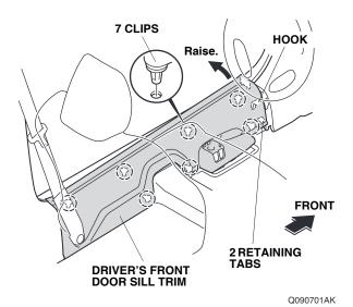
19. Pull away the door opening seal, and remove the driver's kick panel (two clips).
