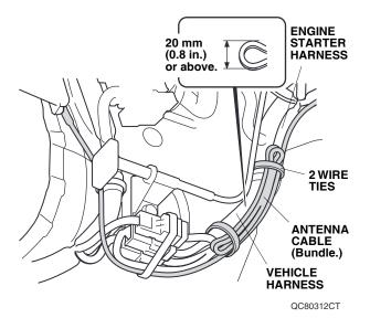
58. Using two wire ties, secure the antenna cable and engine starter harness to the vehicle harness.
