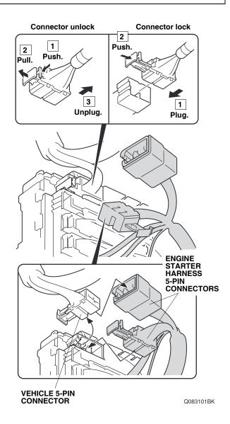
66. Using one long wire tie, secure the engine starter harness 5-pin connector to the vehicle panel.
