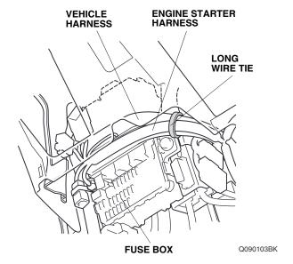
64. Using scissors, cut one urethane tape to the measurements shown. Wrap the cut urethane tape around the engine starter harness 5-pin connector as shown.
