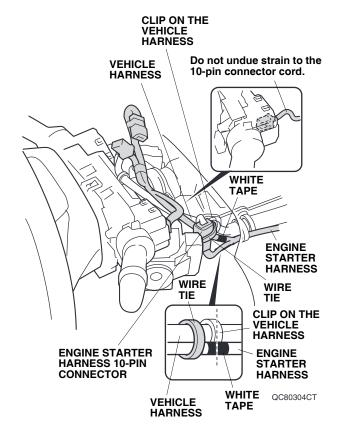
76. Route the engine starter harness as shown. Unplug the vehicle 12-pin connector, and plug it into the engine starter harness 12-pin connector. Plug the remaining engine starter harness 12-pin connector into the combination light switch.
