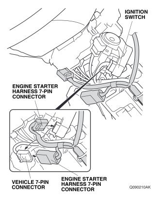
73. Using one wire tie, secure the 7-pin connector and engine starter harness to the vehicle harness.
