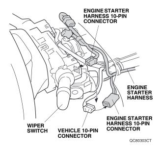
75. Align the white tape on the engine starter harness with the clip on the vehicle harness, and secure the engine starter harness 10-pin connector to the vehicle harness with one wire tie.
