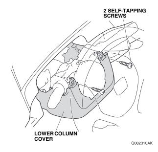
26. Remove the lower column cover (one self-tapping screw).
