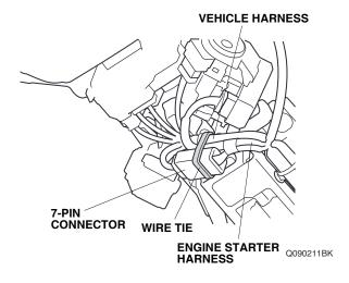
74. Route the engine starter harness as shown. Unplug the vehicle 10-pin connector, and plug it into the engine starter harness 10-pin connector. Plug the remaining engine starter harness 10-pin connector into the wiper switch.
