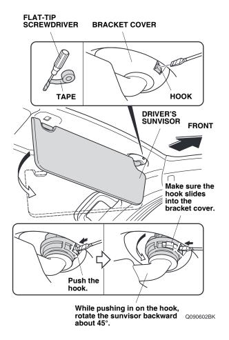
8. While pushing in on the hook, rotate the driver's sunvisor backward about 45°. Make sure the hook slides into the bracket cover.
