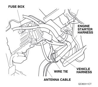
57. Bundle up the excess antenna cable as shown.
