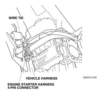
63. Using one long wire tie, secure the engine starter harness to the vehicle harness.
