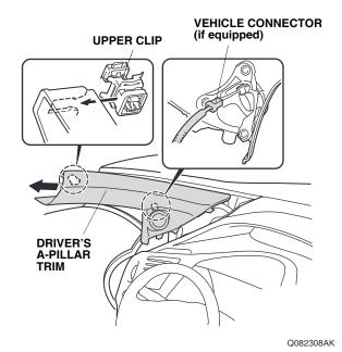
14. Remove the remaining upper clip from the driver's A-pillar.
