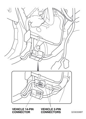
51. Unplug the vehicle 14-pin connector, and plug it into the engine starter harness 14-pin connector. Plug the remaining engine starter harness 14-pin connector into the vehicle 14-pin connector.
