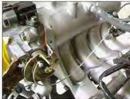
If you use an OEM throttle cable, you'll find that it attaches to the pedal assembly, firewall, and throttle body all in an OEM fashion.
