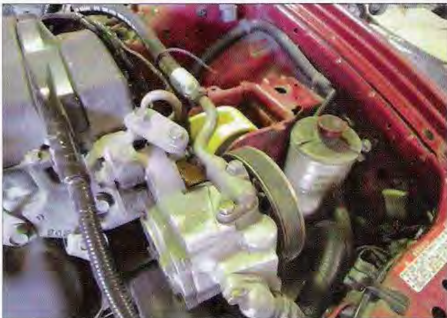
If you have a custom feed line fabricated, the original Prelude power steering components from the donor engine can be installed for a perfect fit.
