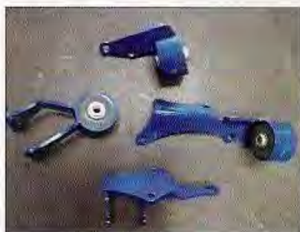
Anytime you're doing a swap as custom as this, you'll need some aftermarket mounts such as these from Place Racing. OEM mounts cannot be used for these B-series transplants unless you want to do some cutting and welding.
