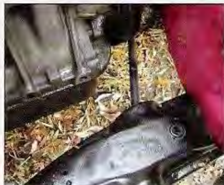
You need to install the Place Racing radius rods in conjunction with their crossmember. The OEM crossmember and rods will hit the crankshaft pulley.
