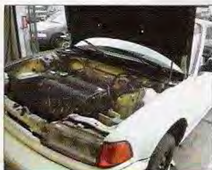
A perfect fit. The ZC engine sits underneath the hood of this Civic in the exact same spot as the old D series.
