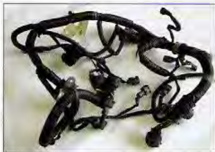
You need to make several modifications to the engine wiring harness. Once the harness is removed from the original engine, you can lay it out on your workbench and take care of business.
