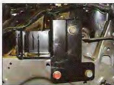
You need to attach the Hasport Performance side mounting brackets to the frame before the engine goes in. It's much easier to do it like this. (Photo Courtesy of Hasport Performance)
