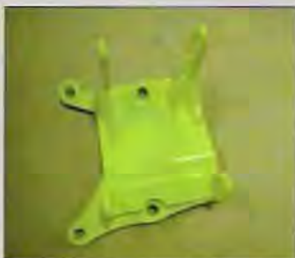
This bracket is designed for the use of an '86-'89 Accord compressor mated to a B series engine.
