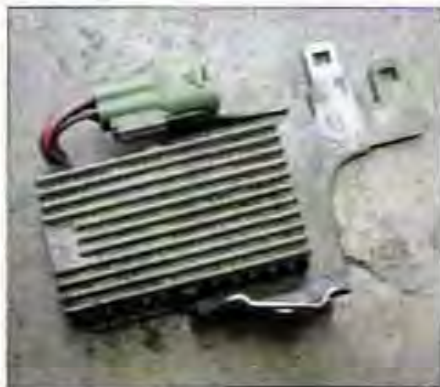
As with most Prelude swaps, you need to add a resistor box since these Civics aren't equipped with one. This 10-year-old Civic resistor box will work just fine.
