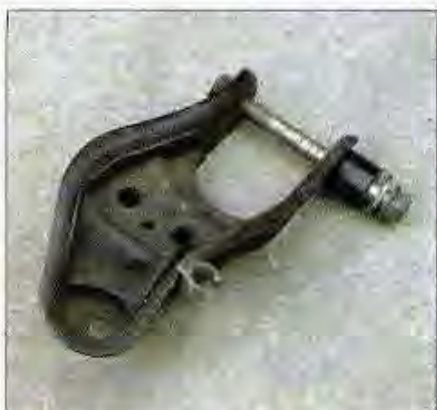
This rear engine bracket taken off of the Civic transmission can be reused regardless of the transmission type. The original Civic and ZC transmissions will both bolt up to the OEM rear mount by using this bracket.
