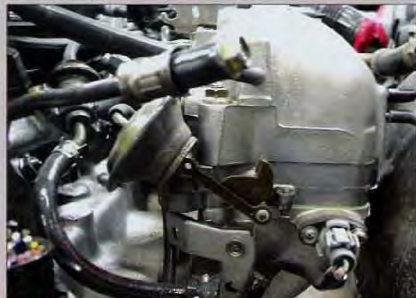
Notice the stacked manifold design. These secondary-type intake manifolds are actually three pieces bolted together.
