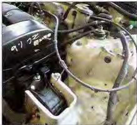
The ZC engine will sit perfectly underneath the hood if you use the appropriate OEM Civic mount. Both the engine mount and the pocket mount remain unaltered when installing the ZC.
