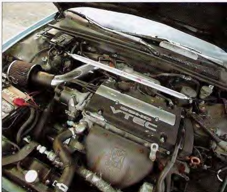
From this angle, you would be hard pressed to tell that an engine swap has even been done. That's one of the nice things about the Accord chassis and Prelude engines.
