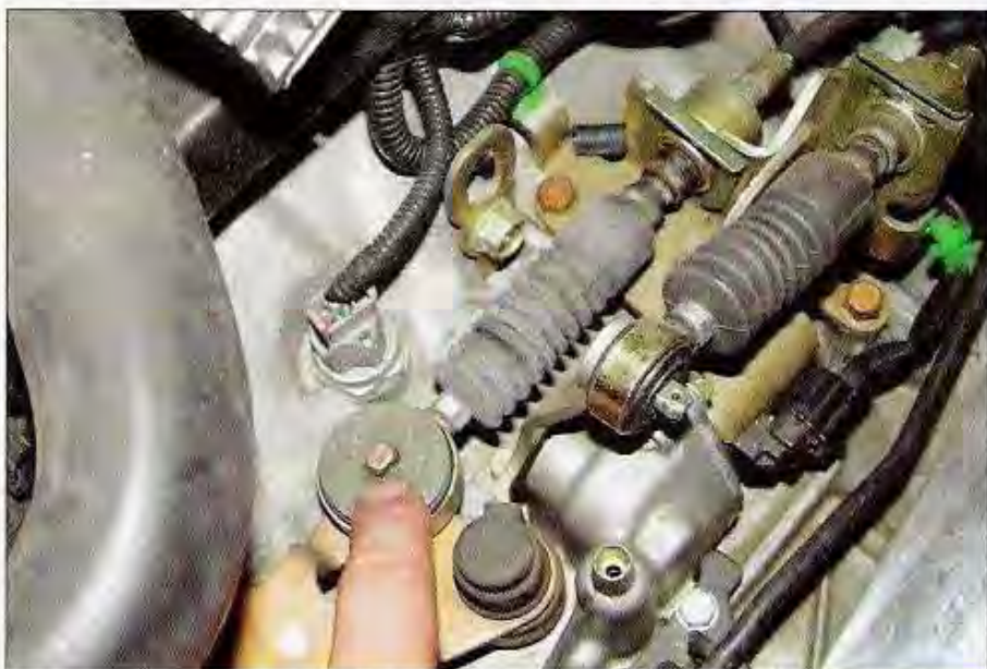
These Civic shifter cables attached to the K-series gearbox in factory form. All of the washers and cotter pins were reused for a perfect fit. (Photo Courtesy of Hasport Performance)
