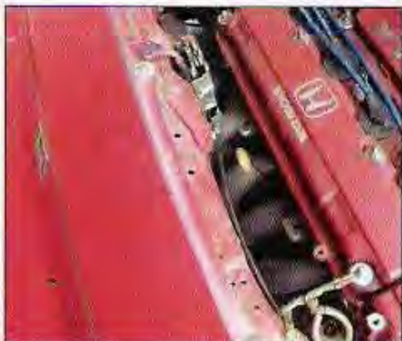
There aren't any clearance issues around the engine bay. Notice the JDM Integra Type R tubular exhaust manifold tucked away.
