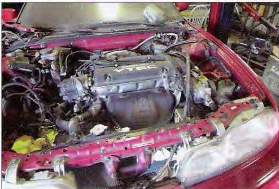
Surprisingly, this is a very nice fit. Thanks to the bolt-in kit from the engineers at Place Racing, second-generation Prelude owners can now have H-series power without too much difficulty.
