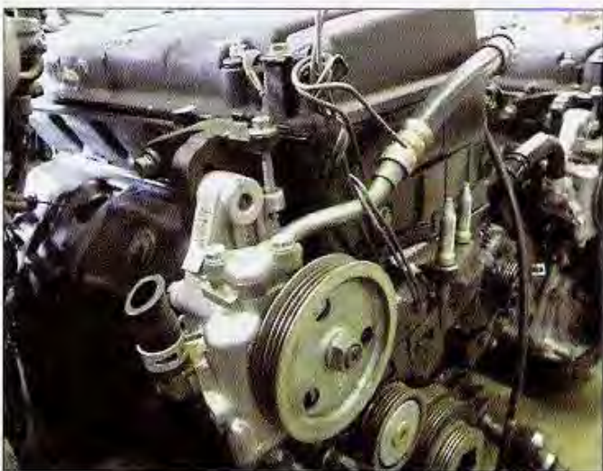
When purchasing a donor H-series engine, be sure to find one with the proper power steering components. You'll need these to make the Prelude line work with the H-series pump.
