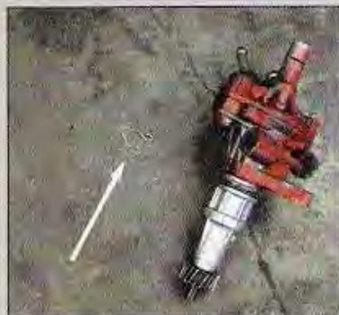
The clip pictured to the left will slip into the groove on the top of the vehicle speed sensor shown on the right. Without it, the cable will slip out of place.
