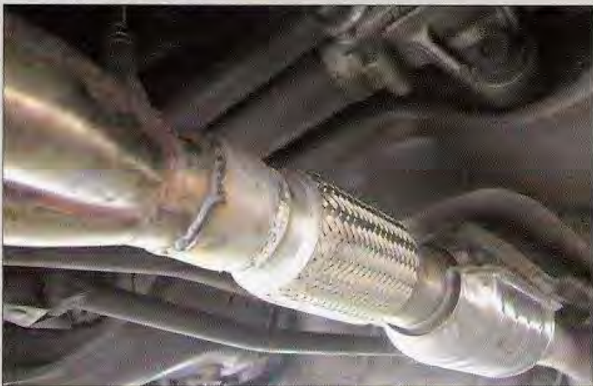
An alternative to the spring-loaded bolts, flex pipes such as these are often times the only option if a much larger exhaust pipe diameter is being used.
