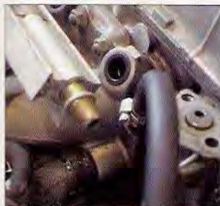
The aluminum sealing washers on the fuel rail should always be replaced when they're removed. The smallest of fuel leaks can pose the biggest problems.
