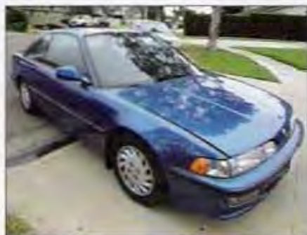
This base-model Integra features the 140-horsepower B18A engine. Although not the most powerful, it is at least a DOHC and worthy of upgrades.
