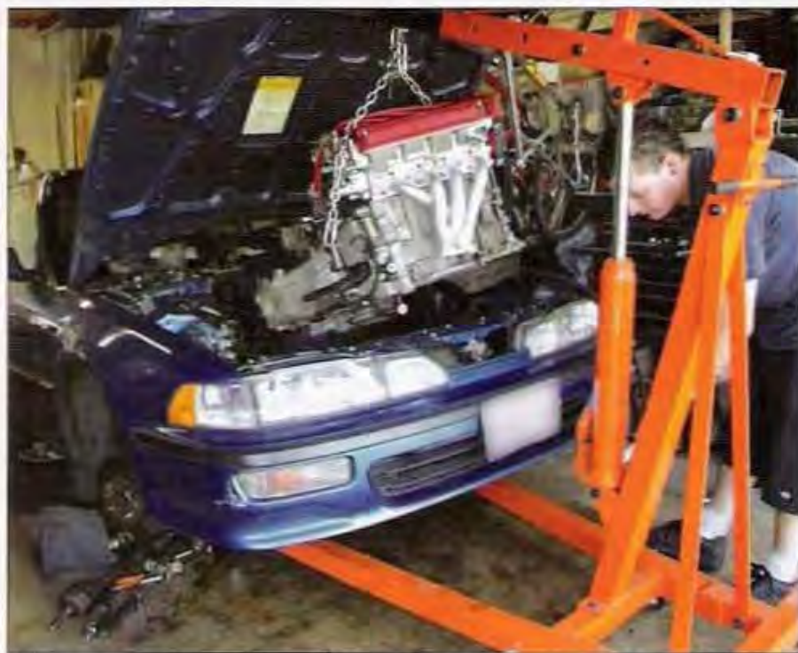
B-series swaps into the second-generation Integras are among the easiest. Robert Young of Holeshoot Racing lowers this B16A in after just a couple hours of work.
