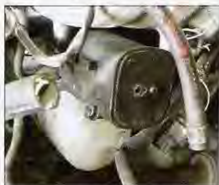
You must use this vacuum box when installing the IAB system for a Prelude engine. Be sure to find one that doesn't have snapped-off vacuum ports like this one (they usually do).
