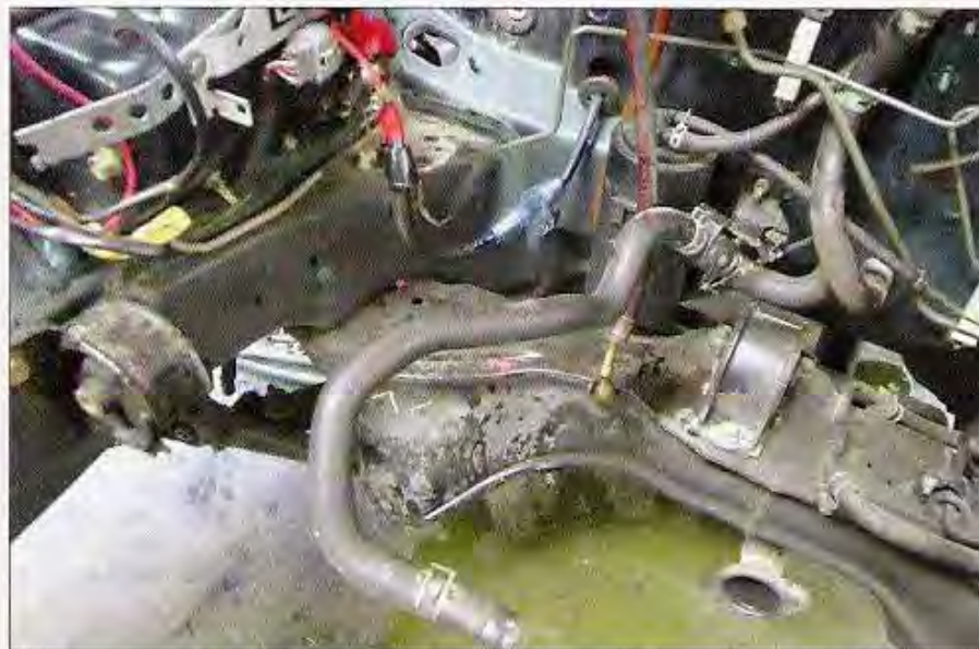
With the B-series swap, this rear mount and heater hose should be left on the vehicle. Since they're going to be reused, don't waste your time taking them off.
