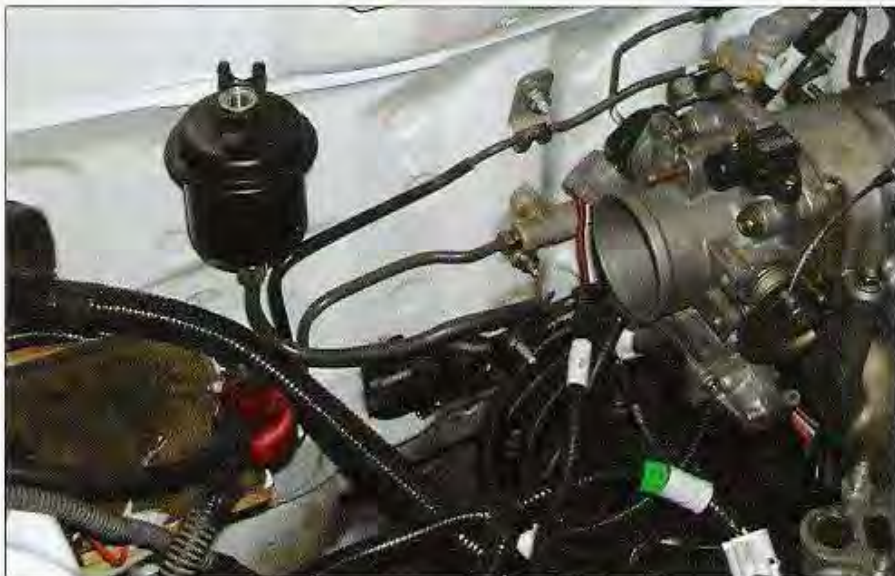
Here's what not to do with the fuel filter. Although it must be relocated, leaving it dangling like this is dangerous and could cause a real problem. At the very least, fasten it down with a large zip tie.
