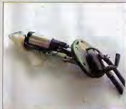
This Civic fuel pump can be replaced with a high-performance unit by simply removing it from the housing that it is mounted to and slipping a new one into its place.
