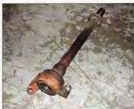
The half shaft you choose will determine which axles you'll need. The female end of this intermediate shaft determines what axle to look for.
