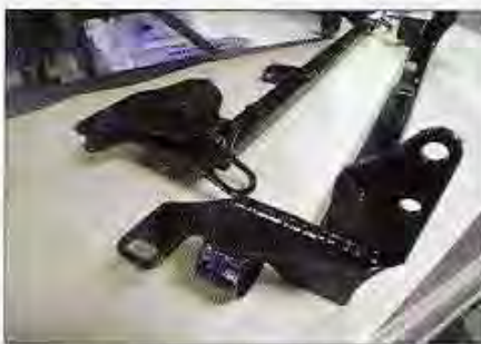
Both of these crossmembers are designed for the '88-'91 Civic from Place Racing. The unit on the right is much more stout and is designed specially for swaps with an H-series engine.
