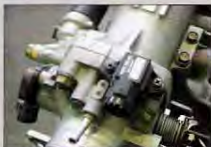
This is a late-model MAP sensor assembly attached to the throttle body. Some other models have their MAP sensors on the firewall.
