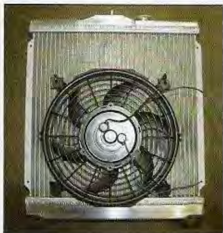
This aftermarket Koyo aluminum radiator and Hayden fan will keep the new H engine plenty cool. If choosing a Honda unit, avoid any radiators that are not twin core in design.
