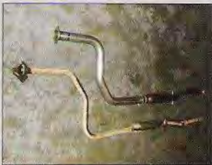
The best place to cut these exhaust pipes would be just in front of the first bend (toward the right in the picture). If you cut too far back, you might mess up the alignment of exhaust hangers.
