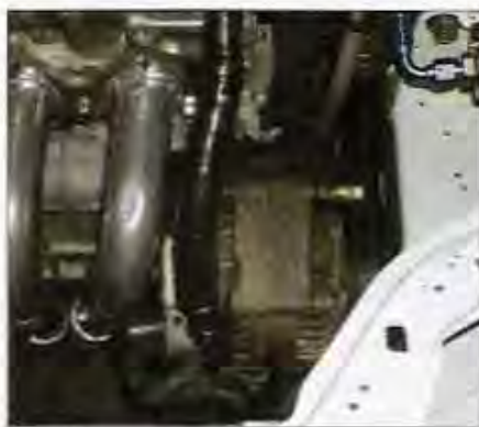
By retrofitting the Prelude alternator wiring onto the Civic or Integra harness, the wires may wrap over the valve cover and down to the alternator. We added some tape and loom to this portion to clean it up.
