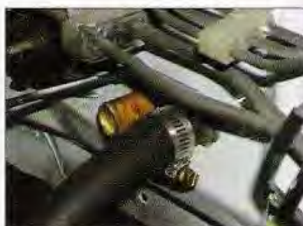
You might want to install this heater hose before installing the H engine. It's tough to get back there once the rear bracket and intake manifold are sitting right in your way.
