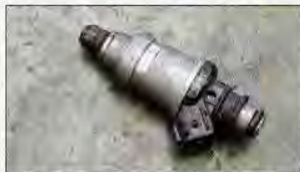
On the dual-injected Civics, two additional injectors must be added inside the engine wiring harness of the vehicle receiving the swap. The new engine will in no doubt be equipped with four injectors.
