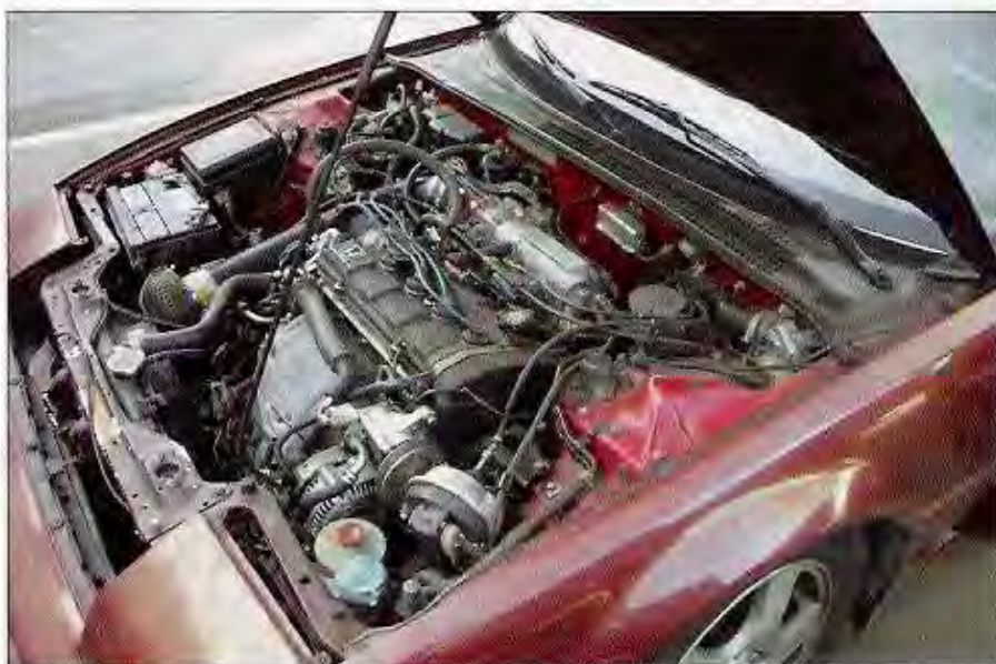
This B20A5 engine is hopeless as far as horsepower is concerned. These engines feature a composite head gasket as opposed to the standard metal version, so they can't withstand much horsepower.
