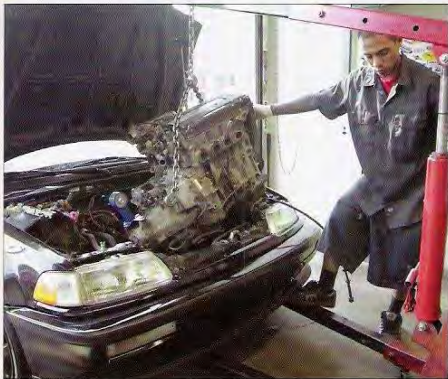
Eric Cardines of Honda Fiend installs this early model B16A engine into a fourth-generation Civic hatchback with the help of a set of Place Racing engine mounts.
