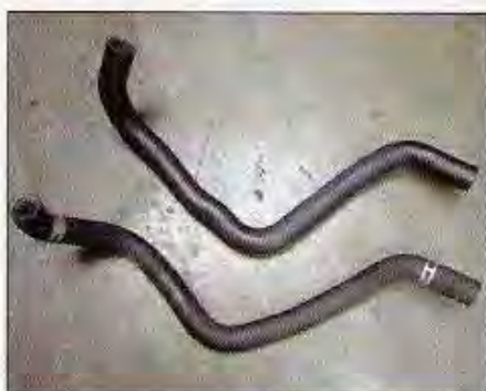
The newer Integra radiator hose featured on top is slightly larger in diameter compared to the Civic and Integra hose. The hose must be tightly clamped down to the radiator neck because of its larger size.
