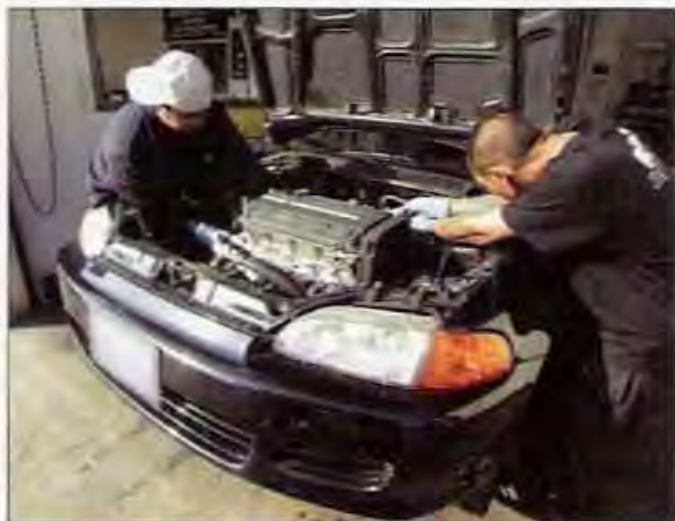
The crew at Honda Fiend works together to make short work of this B18C GSR swap into a fifth-generation Civic Si.
