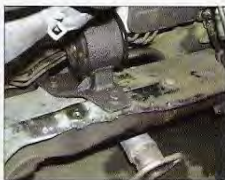
This HCP Engineering rear engine mount has been bolted into place after the rear crossmember lip was pounded down flat. It's better to flatten it too much than not enough so that the bracket won't fit.
