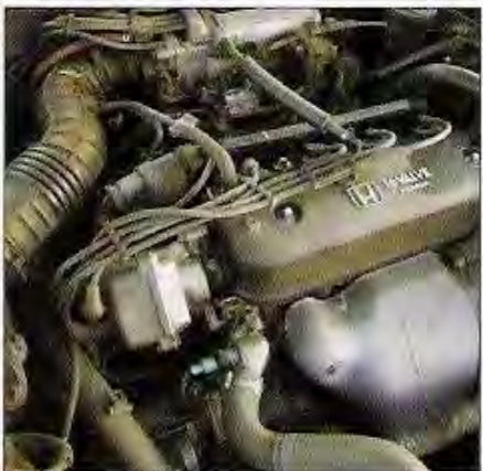
The featured SOHC F-series engines aren't the best engines to modify, especially considering how easy it is to install a DOHC H series.
