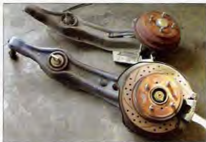
Rear brake conversions on the '88-'91 Civic are a breeze, thanks to the Integra. The trailing arms are nearly identical so they'll simply bolt into place.
