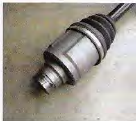
Late-model Integra axles are generally used on these swaps even though several other early Integra and custom combinations are possible.
