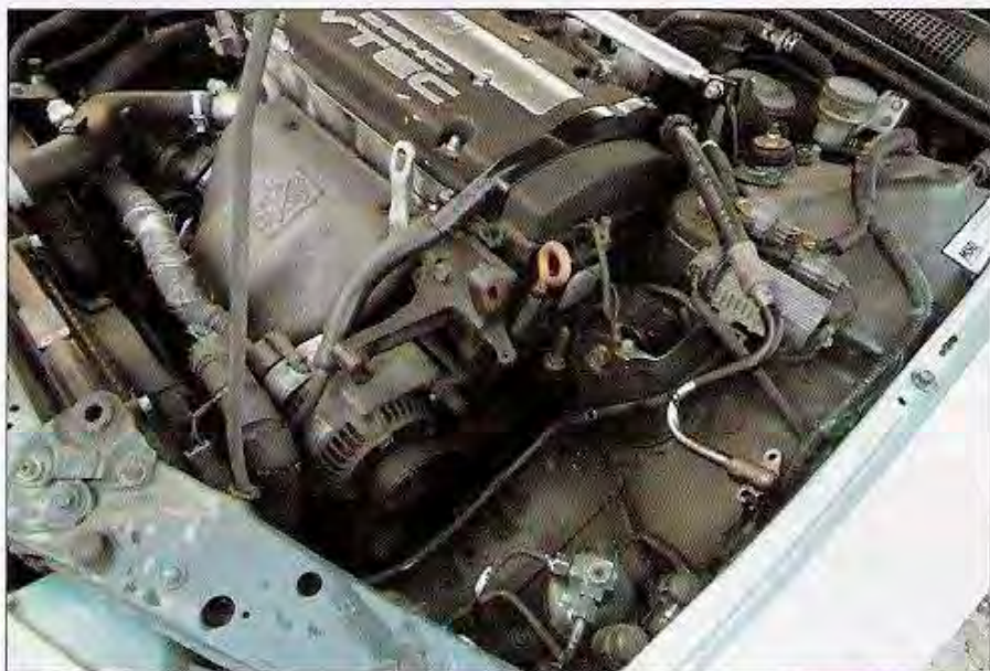
Notice the air conditioning lines running alongside the front of the radiator. There is also plenty of clearance in regards to the cooling fan and the condenser fan as well.
