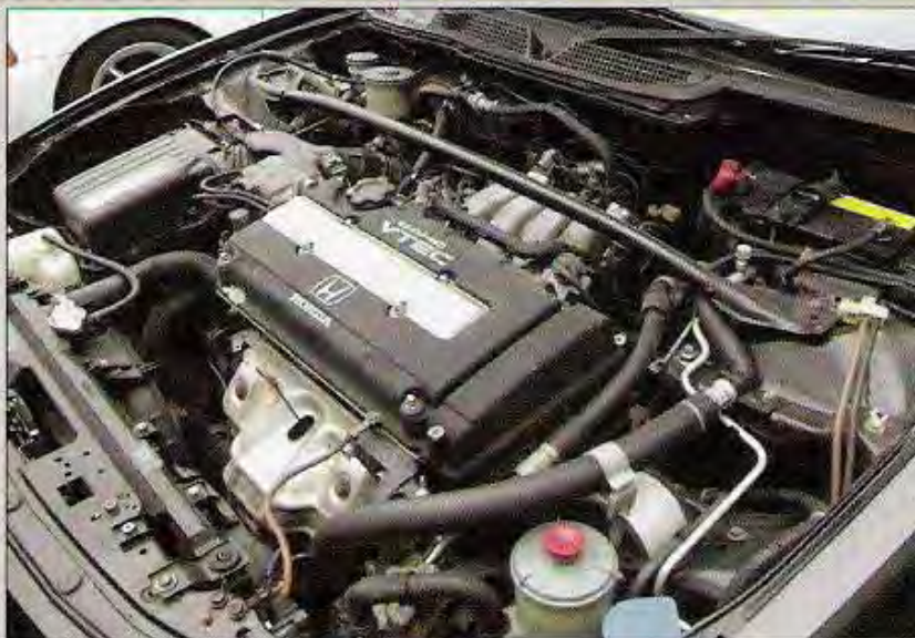
Notice the brake booster, battery, A/C lines, and fuse box are all on the opposite side of the engine compartment.
