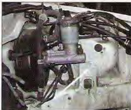
This pocket mount in the middle right of the photo must be drilled out and removed before installing the specialized bracket from Place Racing.
