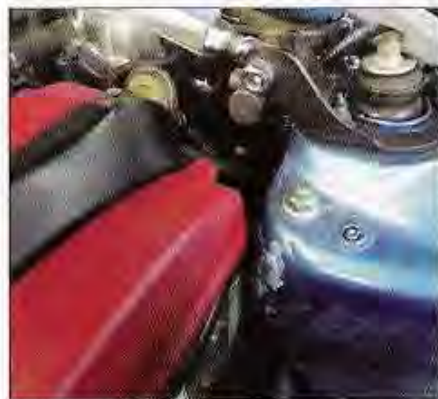
Notice how close the engine sits to the shock tower of the Integra. You can get plenty of clearance by cutting the valve cover off on the end.
