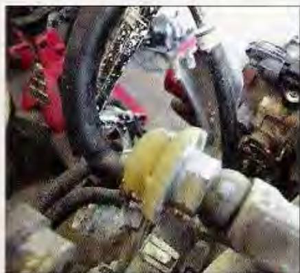
Removing this fuel dampener pulsation cap with a 22-mm wrench will allow you to install the Civic fuel injection feed hose. Be careful not to over tighten this cap.
