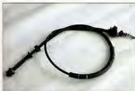
This right-hand drive throttle cable is way too long. It would need to wrap clear around the engine, and it won't sit properly. Be sure to install the proper USDM throttle cable.
