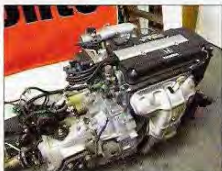
OBD II B16A engines make a perfect donor engine for this chassis, as it's totally compatible in terms of mounts and electronics. This one is from a Civic Si.
