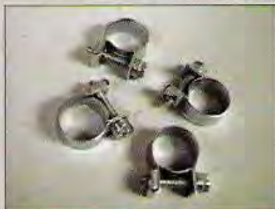
Notice how these fuel-injection hose clamps don't have the ridges in them that you would normally find in a standard hose clamp.
